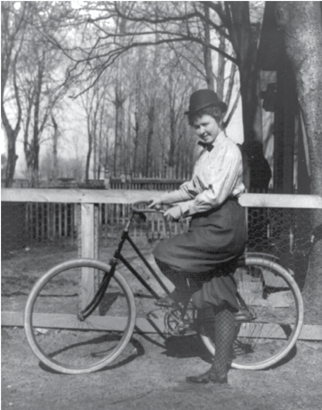
A woman wears comfortable riding pants, and the bicycle has a lowered or “safety” cross bar for easier (and more modest) swing-of-the-leg dismounting, ca. 1897.
